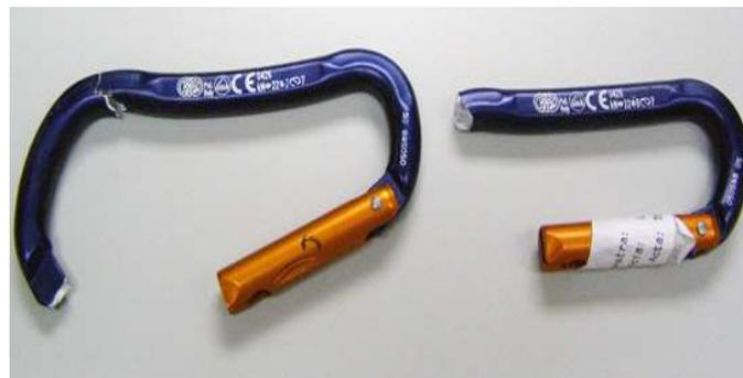
The product poses a risk of injuries because it does not withstand the static strength test which could lead to falls. The test was carried out on the major axis, and it was noted that the connectors break when the following forces are applied:
