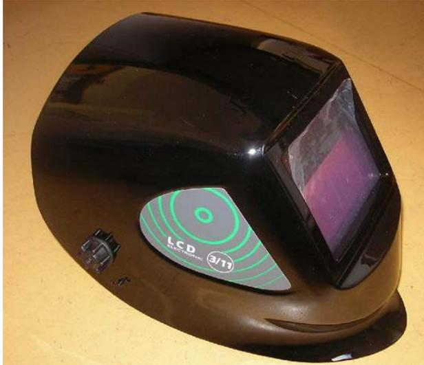
When the welding arc is ignited, the filter switches its protection stage automatically from low (bright state) to high (dark state).
