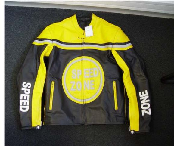
The product poses a risk of injuries because after a series of three impacts, each one the equivalent of 50 Joule, the average force registered under the anvil is much higher than the maximum permissible limit (a maximum of 24770N for 18000N). The back protection even cracked after the third impact, therefore making it impossible to carry out all five impact tests required by the standard.
